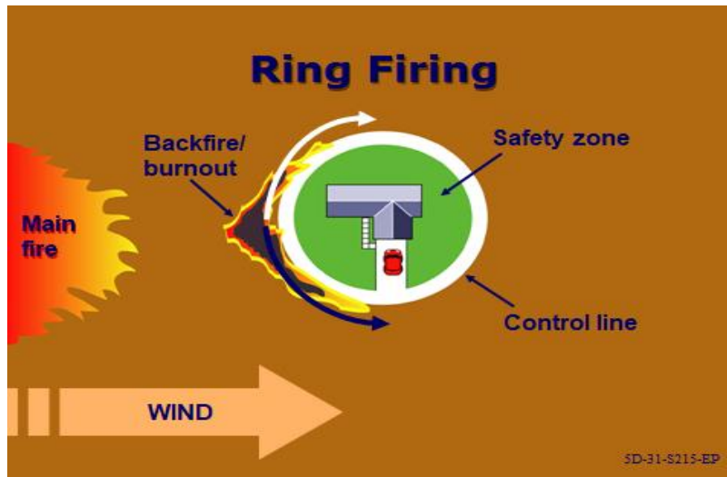
Figure 6 Ring firing method
