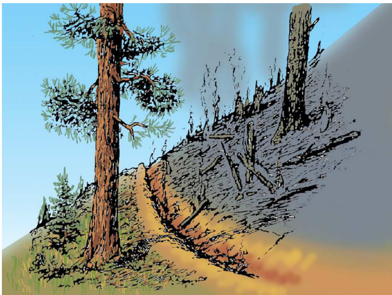
Figure 2: “Hot spot” to find and extinguish burning areas close to line
