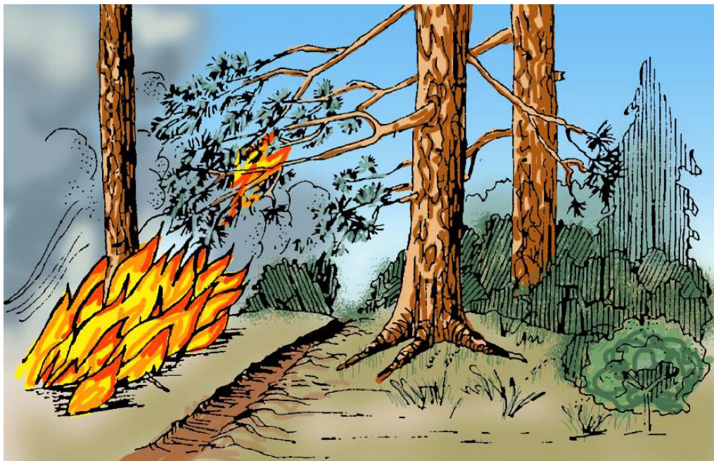
Figure 1: Low-hanging limbs can spread fire across fire Line
